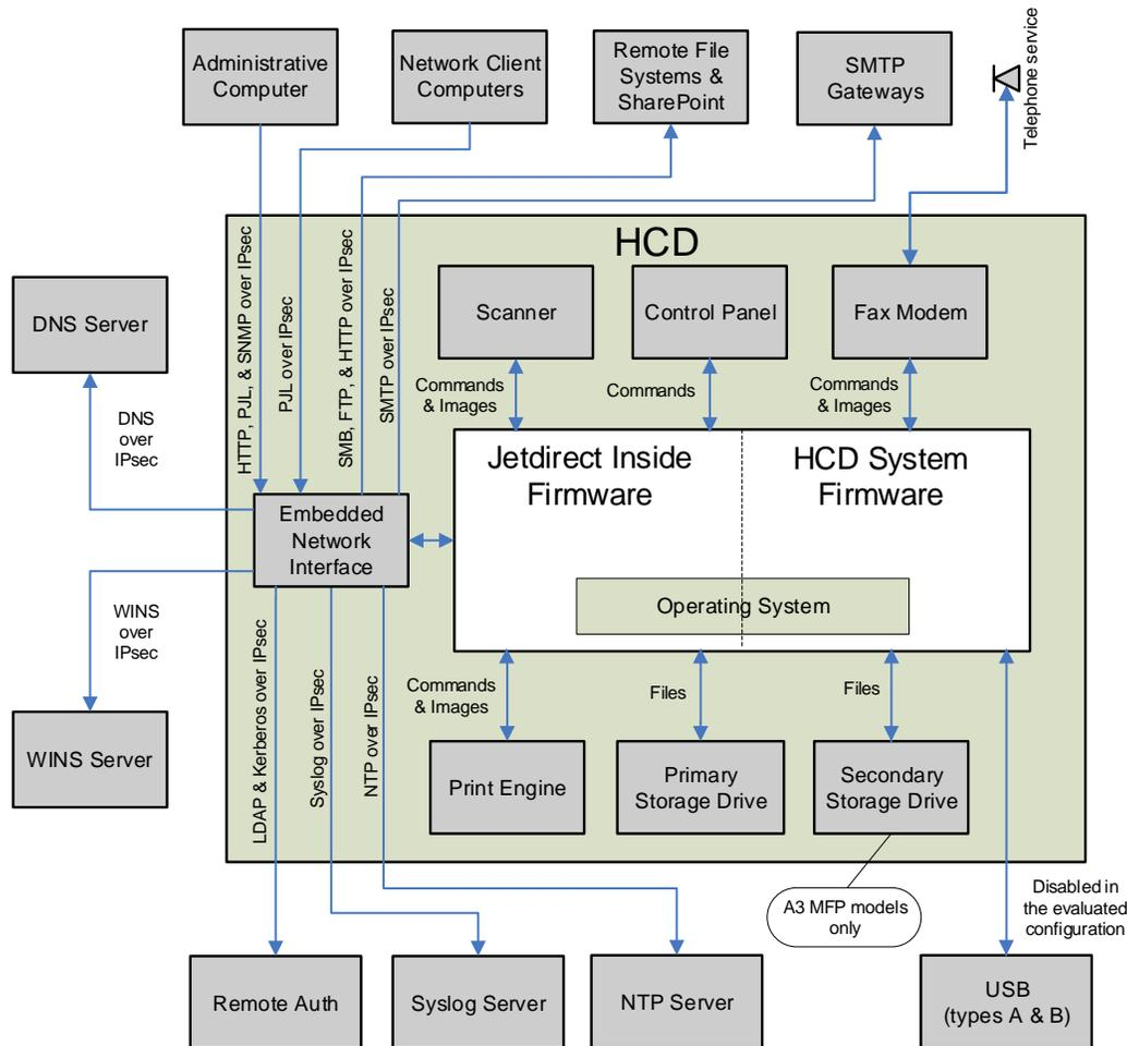
Figure 1 shows a high-level physical diagram of an HCD with the unshaded areas representing the TOE and the shaded areas indicating components that are part of the Operational Environment.
